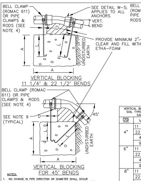
NO CHANGE IN PIPE DIRECTION OR DIAMETER SHALL OCCUR
