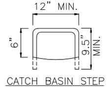
\* ALL STEPS & RUNGS #8 GALV. DEFORMED REBAR OR POLYPROPYLENE.
