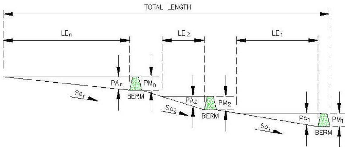
**Figure 6.2. Schematic for calculating Bottom Length and Effective Total Depth for bioretention or pervious pavement on slopes where check dams (berms) are used. Refer to Table 6.6 for Rain Gardens and Bioretention Swales, and Table 6.8 for Pervious Pavement formulas.**
