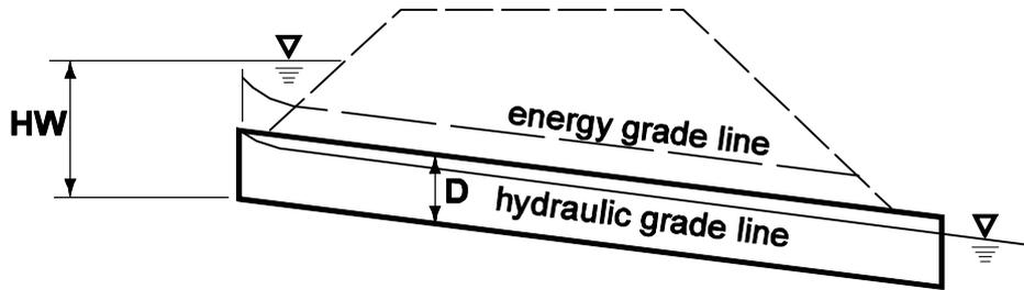
**Inlet Control - Submerged Inlet**
