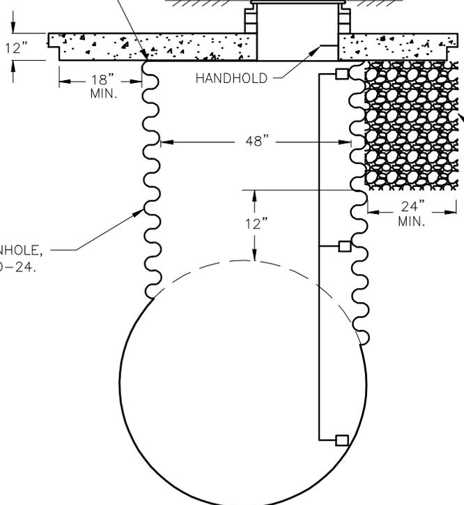
CRUSHED SURFACING TOP COURSE PER WSDOT STD. SPEC. 9-03.9(3). COMPACT TO 95% MAX. DENSITY PER ASTM D1557.
