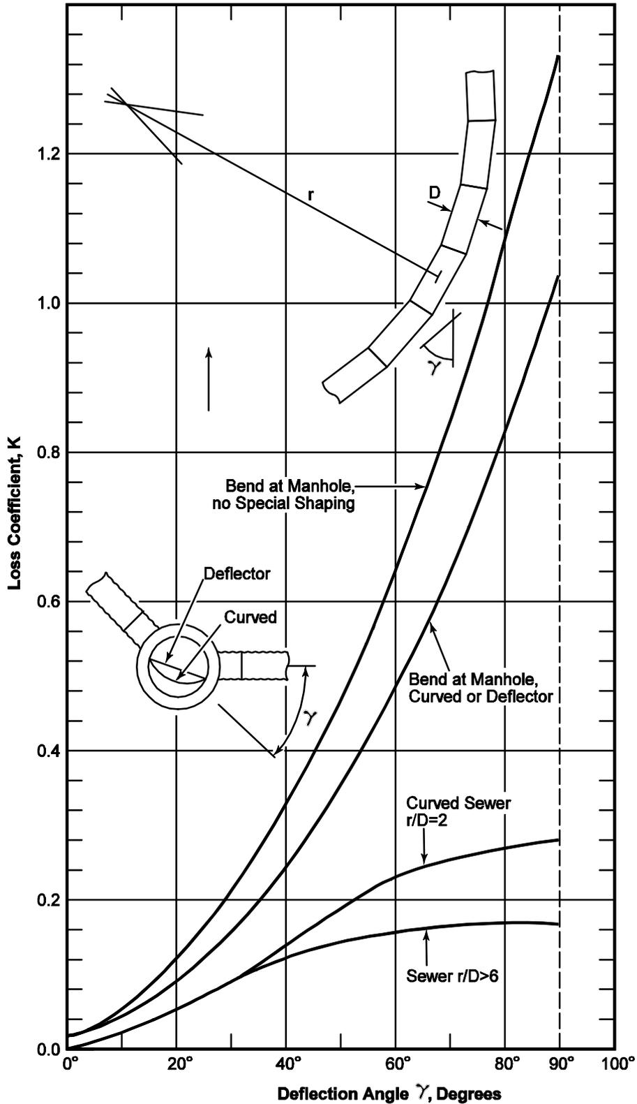
Figure 4.21 Junction Head Loss In Structures
