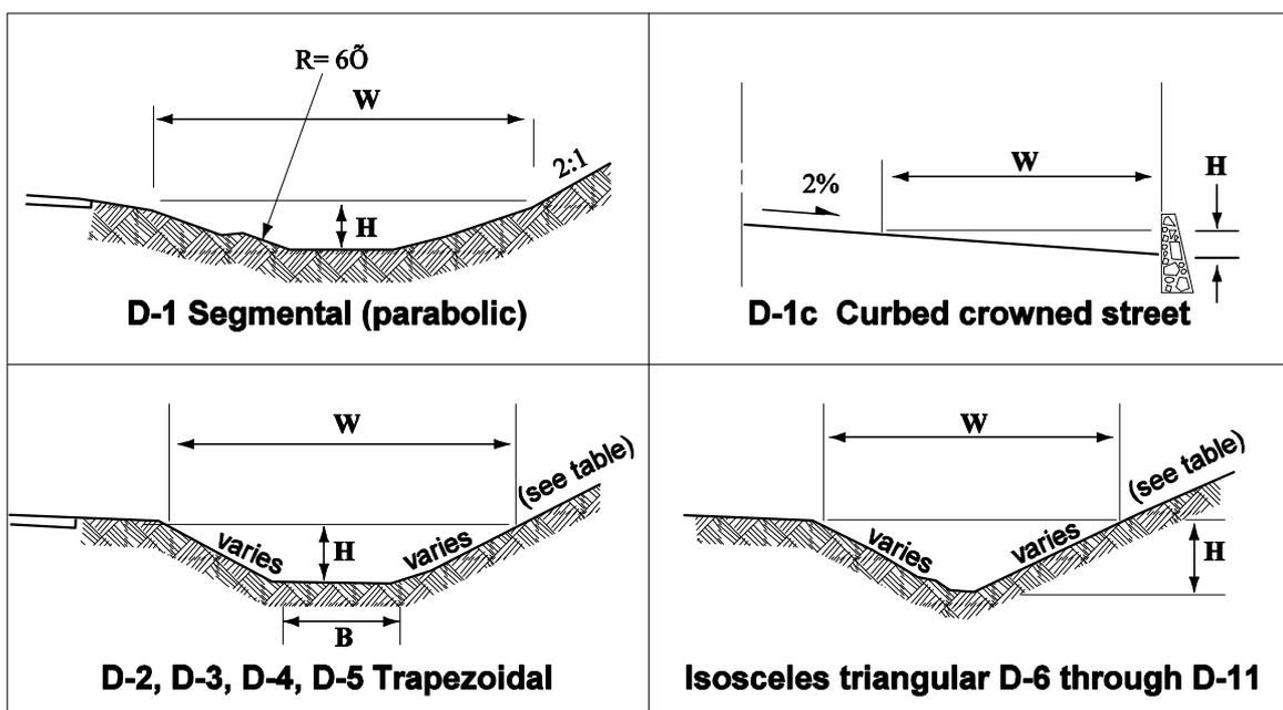
**Figure 4.4 Drainage Ditches - Common Sections**
