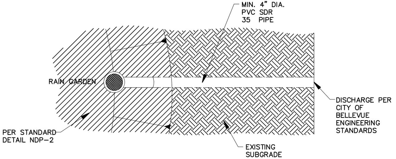
SECTION A – RAIN GARDEN OVERFLOW WITH PIPE CULVERT
