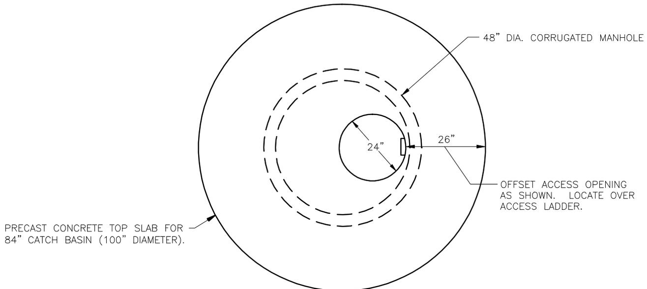
PRECAST CONCRETE TOP SLAB FOR 84" CATCH BASIN (100" DIAMETER).
