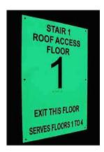
The International Fire Code sets forth minimum requirements for maintaining the life safety of building occupants. In this instance, stairwell identification signs are required at each floor landing in new and existing buildings with interior exit stairways and ramps connecting more than three stories. The intent of this requirement is to make signs visible and immediately recognizable to building occupants and emergency responders using the stairway.
