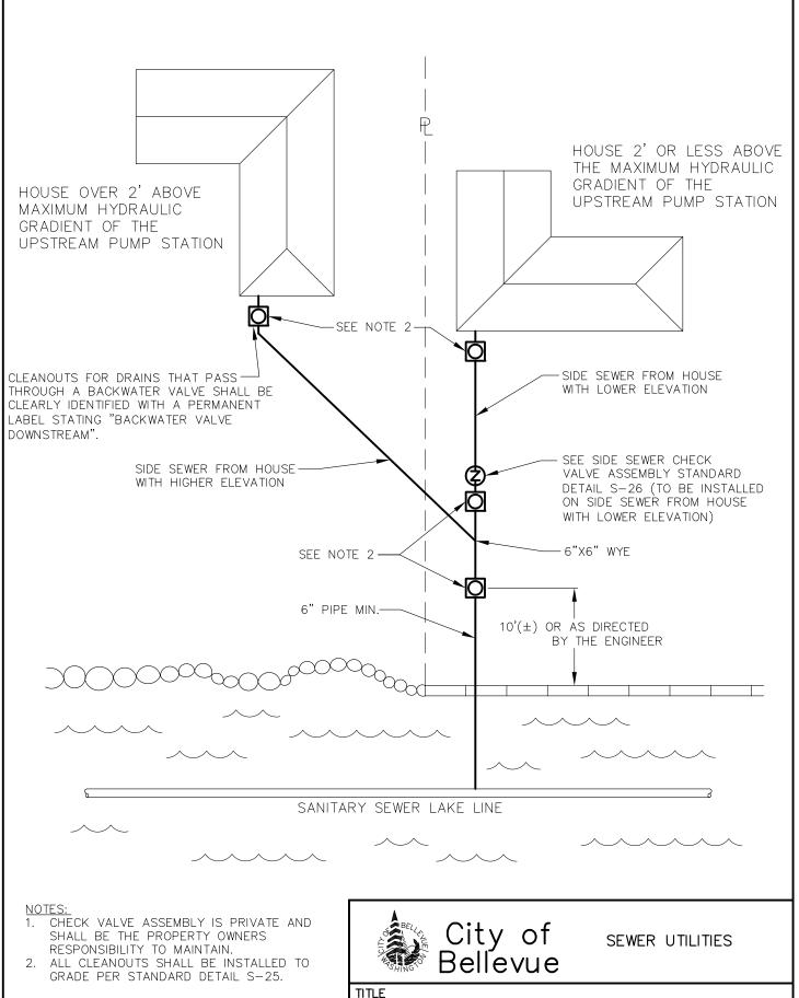
LAKE LINE CLEANOUT AND CHECK VALVE ASSEMBLY INSTALLATION
