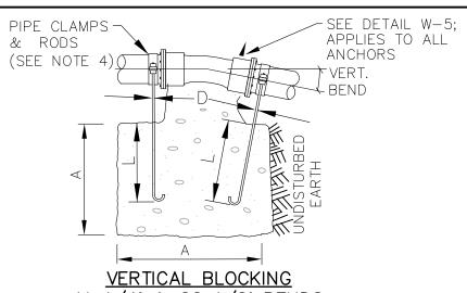
PIPE CLAMPS -& RODS (SEE NOTE 4) O.D 90° ⋖ COMPACTED BACKFILL (SEE NOTE 7) VERTICAL BLOCKING FOR 90° BENDS
