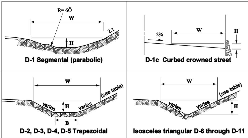
**Figure 4.4 Drainage Ditches - Common Sections**
