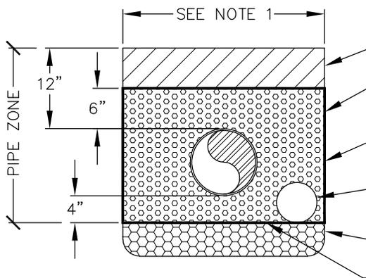
DETENTION PIPES WITH UNDERDRAINS
