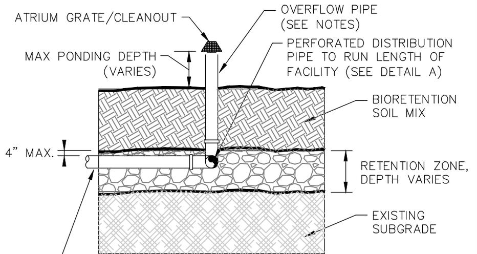
BIORETENTION WITH UNDERDRAIN
