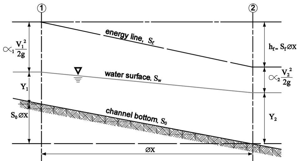
$$S_o \Delta x + y_1 + \alpha_1 \frac{V_1^2}{2g} = y_2 + \alpha_2 \frac{V_2^2}{2g} + S_f \Delta x \quad (4-1)$$
