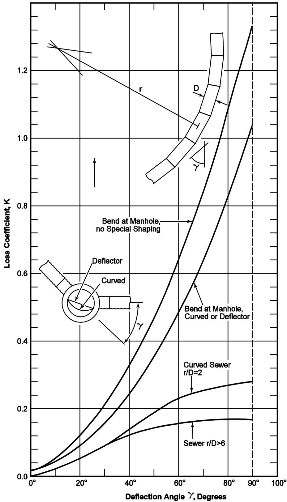
Figure 4.21 Junction Head Loss In Structures
