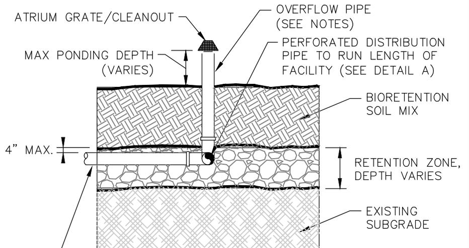
BIORETENTION WITH UNDERDRAIN
