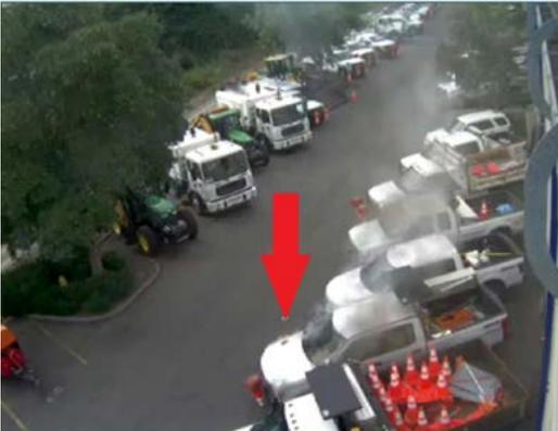
**August 20, 2019** – Security footage captured the first signs of smoke. Fire began to engulf the vehicle as Bellevue Fire arrived on scene. The fire caused an estimated \$174,236 to 3 vehicles and the adjacent building. It was determined to be related to failure of electrical components in the engine compartment.
