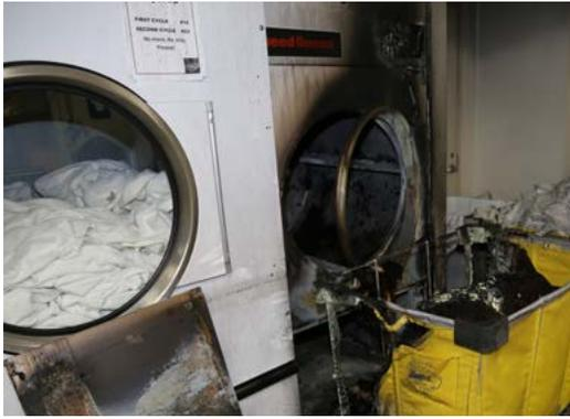
**October 10, 2019** – A commercial dryer caught fire shortly before midnight. The fire department was alerted by a water flow alarm after the adjacent fire sprinkler head activated.
