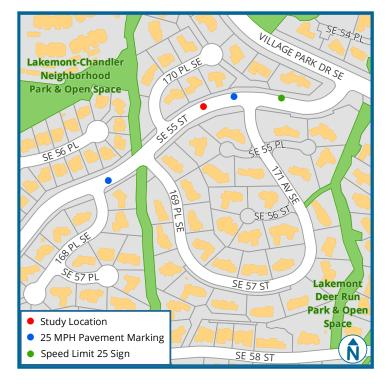
You specifically were concerned about vehicle speeds on SE 55th Street. The roadway grade on SE 55th Street is too steep to meet our guidelines for the installation of speed humps.
