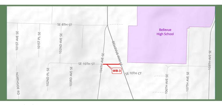
**Description:** This project would install a new sidewalk and marked crossing on SE 10th St between SE 104th SE to Bellevue Way SE, connecting a gap in the sidewalk network. The sidewalk would replace the existing gravel shoulder, **eliminating approximately six (6) parking spaces**.
