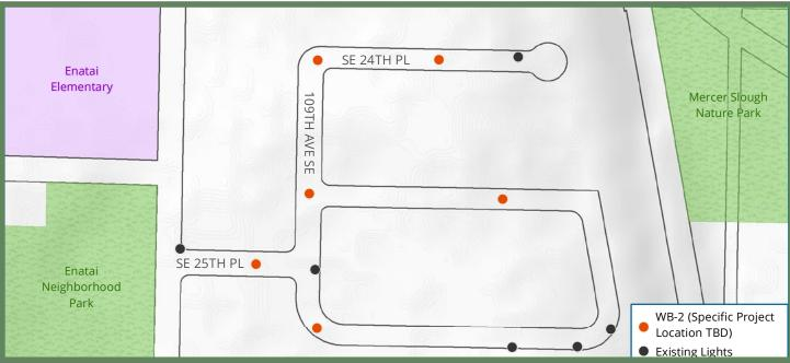
Description: This project would install up to six (6) new LED street lights in the Bell Forest area. New street lights would be installed on existing PSE wood utility poles. On-going electricity costs would be paid for by the City. Actual locations would need to be examined further with PSE for feasibility. Specific street light locations are to be determined.
