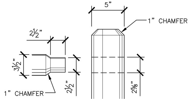
MILLING & DRILLING DIMENSIONS
