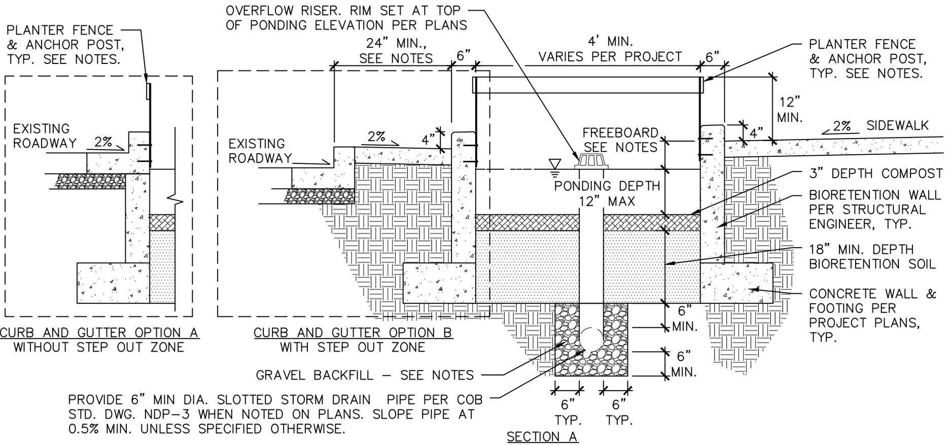
PROVIDE 6" MIN DIA. SLOTTED STORM DRAIN PIPE PER COB STD. DWG. NDP-3 WHEN NOTED ON PLANS. SLOPE PIPE AT 0.5% MIN. UNLESS SPECIFIED OTHERWISE.
