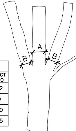
ASPECT RATIO OF B:A GREATER THAN OR EQUAL TO 0.66 AS MEASURED 1" ABOVE THE TOP OF THE BRANCH UNION.
