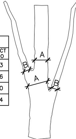
ASPECT RATIO OF B:A LESS THAN 0.66 AS MEASURED 1" ABOVE THE TOP OF THE BRANCH UNION.
