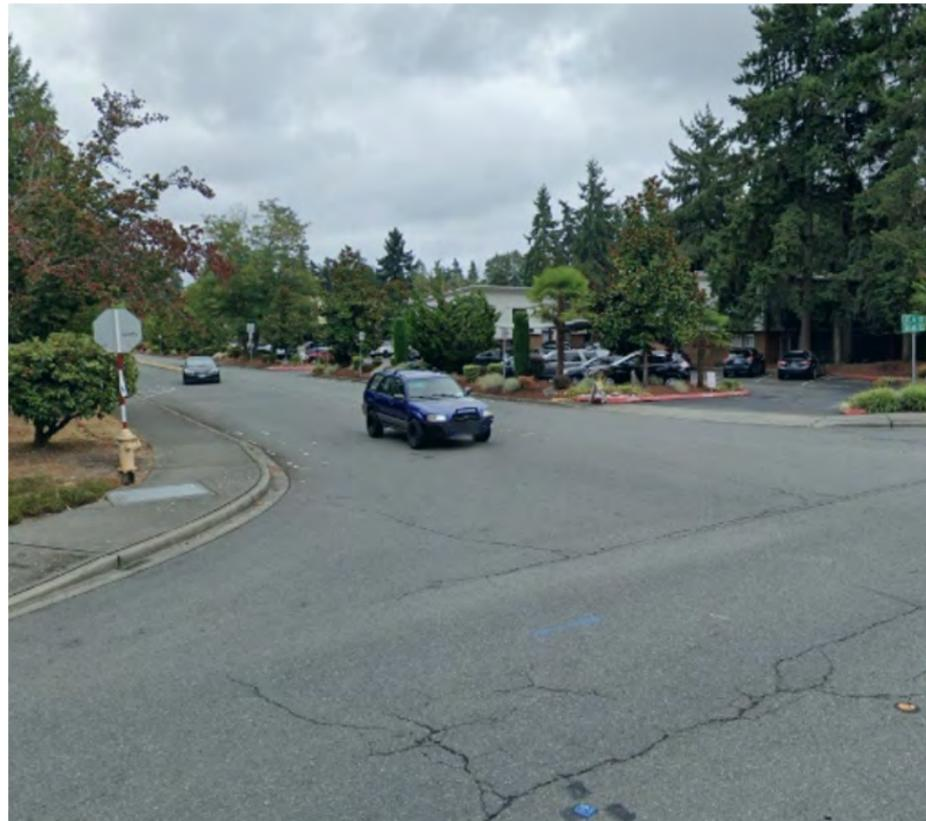
Figure 28: Facing eastbound at the intersection of Southeast 6th Street and 140th Avenue Southeast. Wide intersections with no marked crossings and large turn radii are typical within this RSA area.
