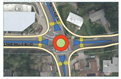
Roundabout has the largest impacts to adjacent properties and driveways, and highest construction cost compared to other alternatives.
