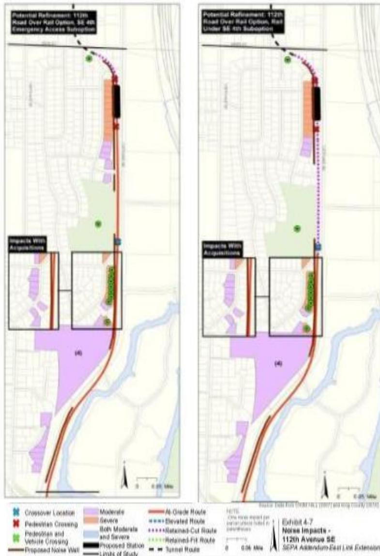
Overall cumulative noise levels lowest with SE 4<sup>th</sup> Emergency Access and highest with Road under Rail
