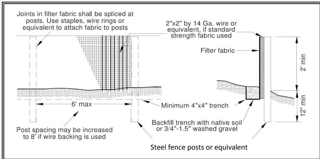
**Figure 4.2.12 – Silt Fence**
