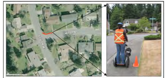
During the sidewalk inventory effort, the City employed a rigorous QA/QC protocol for validation testing of the data results. Field verification of ULIP results involved taking smart level measurements of sidewalk grade every 2 feet over a 70 foot span. Numerous assessments of ULIP data, evaluated at the same interval as the smart level (2 feet), confirmed that the ULIP grade data provides an accurate interpretation of the geometry of the sidewalk profile. The images above reflect the results of a field test of ULIP sidewalk grade at 174th Avenue NE and NE 11th Street.
